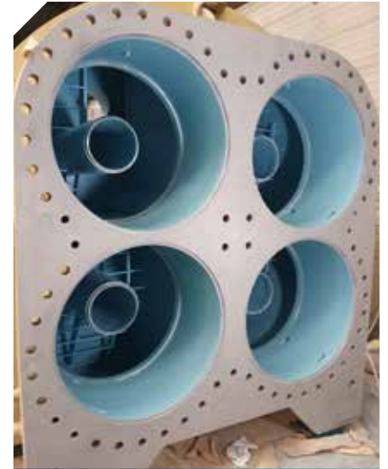
Cooling water area following protective coating
